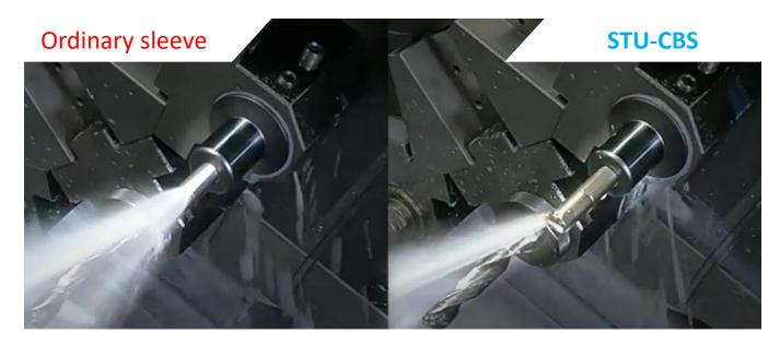
Don't let the coolant escape! Aim the coolant where it needs to be! NT Tool's new and unique design seals coolant 100% and will leads to better machining and longer cutting tool life. YouTube video<u>https://youtu.be/IDFgXsrPCYY</u>
